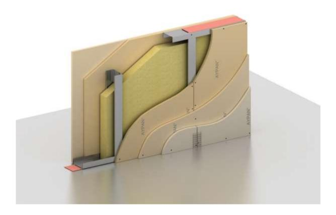
1 TP 23 AYSIST® Partition Wall System is built by screwing three layers of Aypan plasterboard to one side and double layers of Aypan plasterboards to the other side over a metal single framework(DC) as indicated conditions in its technical specifications. The system contains insulation panels (rock wool divisionboard) inside selected in accordance with the length of the wall and the required insulation properties.
