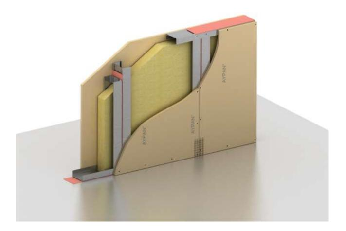
1 CP 11 AYSIST® Partition Wall System is built by screwing Aypan plasterboard to both sides of a metal double framework (DC) as indicated conditions in its technical specifications. The system contains insulation panels (rock wool divisionboard) inside selected in accordance with the length of the wall and the required insulation properties.
